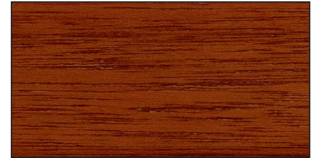
17 Holzart: Meranti Induline SW-900 farblos Belastungs-Gruppe: Induline GW-360 teak B6/III-E Induline LW-700/40 teak
